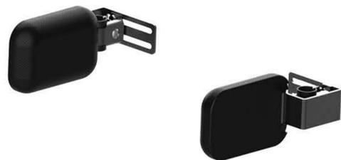
These lateral trunk supports bolt on to the back canes. Each pad is adjustable for depth, angle, height and width. The pads have a 4 x 5 array of holes on the back. Each pad includes a washable fabric cover.
